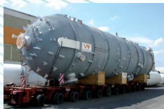
Cracked Gas Dryer
